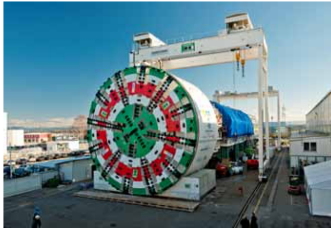
The Herrenknecht S-574 Earth Pressure Balance Shield at the Schwanau plant.
