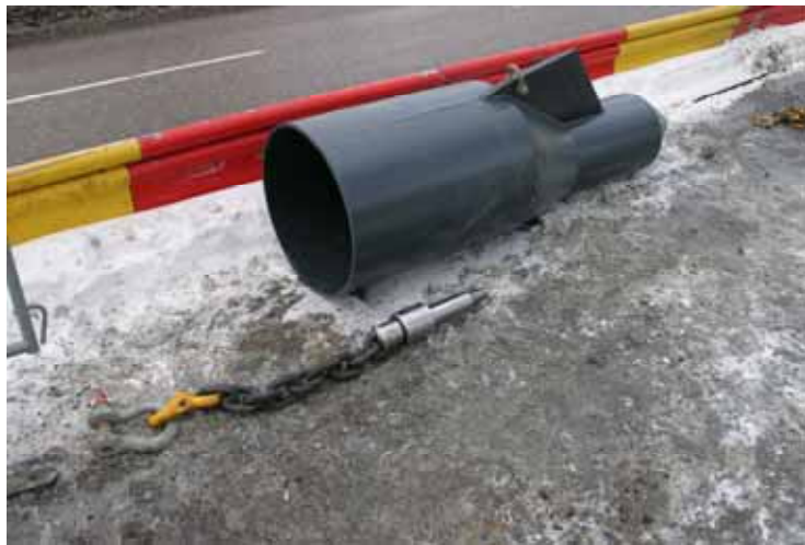
A typical pipe bursting head as used on the recent Gothenburg replacement project.
