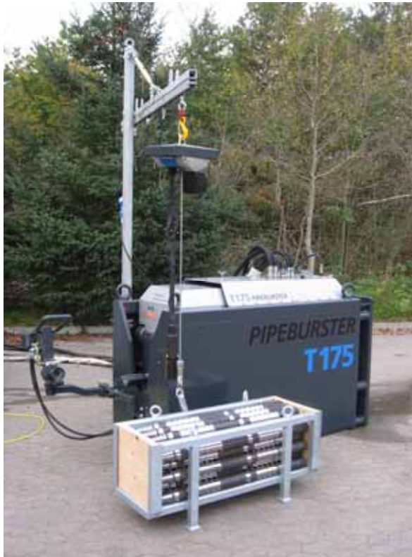
The Scandinavian No-Dig Centre T175 pipe burster recently purchased by Gothenburg Water Board.
