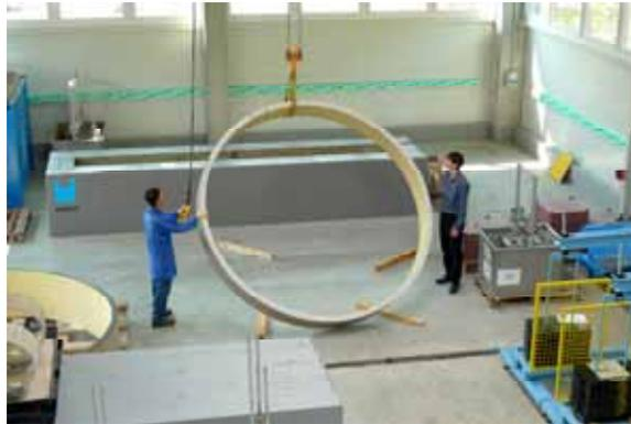
*HOBAS can now conduct in-house tests on pipes of up to 4 m diameter.*
