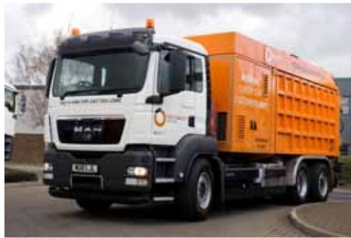
*One of the two new MAN TGS 26.440 6x2-4 BL chassis with ground-breaking suction excavation equipment from TT-UK.*
