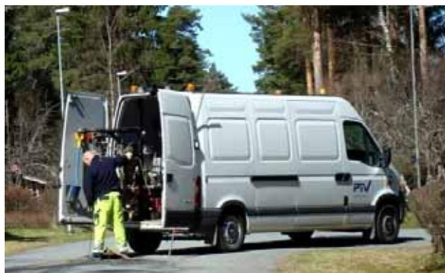
*The DigiSewer<sup>®</sup> unit, mounted in a survey van, being placed into a pipeline prior to a measuring run.*
