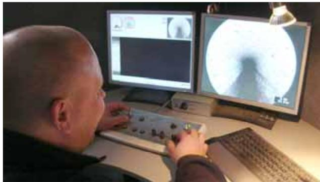
*The operator's survey control desk of the DigiSewer® system showing operational displays.*
