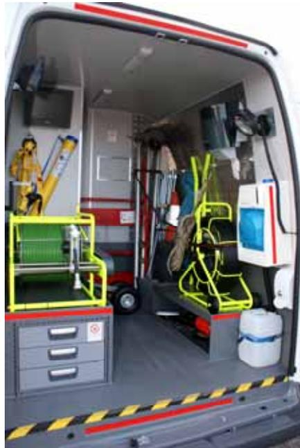
*Both mainline and rod camera systems are easily accessible from the back of the survey van.*
